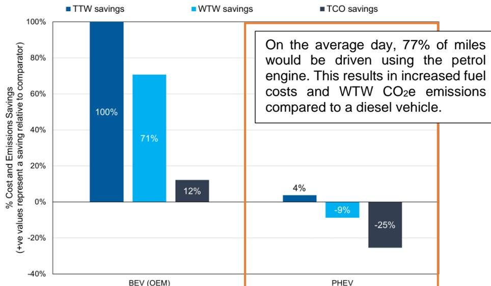
On the average day, 77% of miles would be driven using the petrol engine. This results in increased fuel costs and WTW CO<sub>2e</sub> emissions compared to a diesel vehicle.
