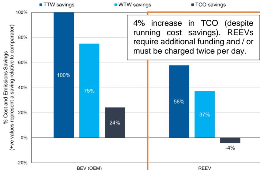
Figure 12 - CO<sub>2</sub>e Emissions Savings vs. Cost Savings; Medium Van (WAV)
