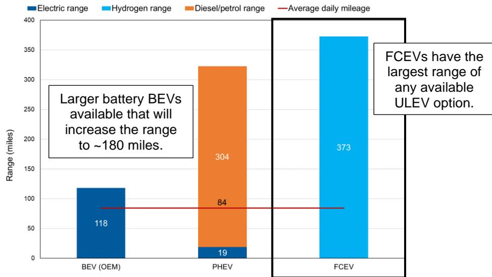
Operating Range; Medium Car, Fuel Cell Electric Vehicle
