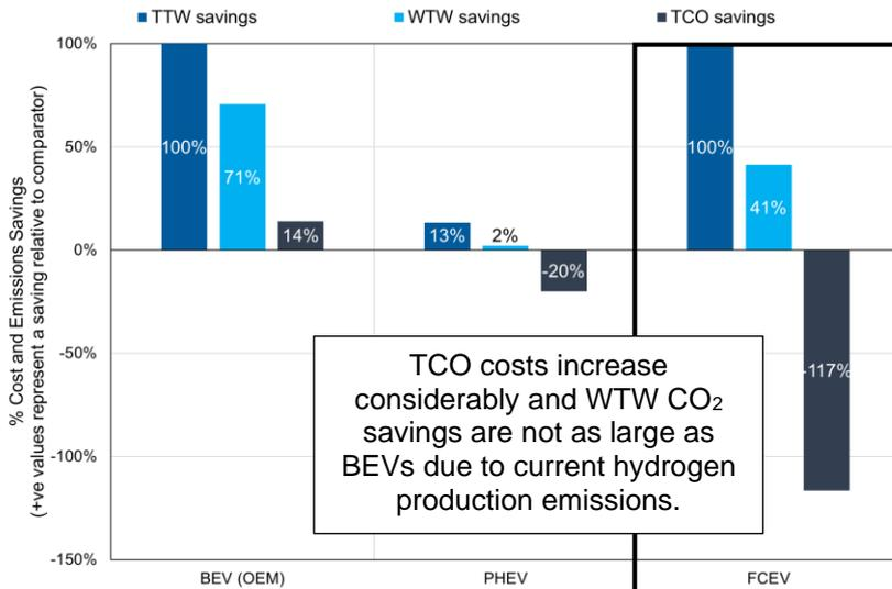
CO<sub>2</sub>e Emissions Savings vs. Cost Savings; Medium Car, Fuel Cell Electric Vehicle
