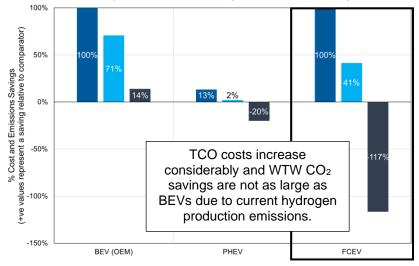
CO2e Emissions Savings vs. Cost Savings; Medium Car, Fuel Cell Electric Vehicle
