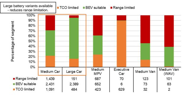
Figure 15 - Detailed Breakdown of BEV Suitability by Vehicle Segment (Standard Battery Capacity)
